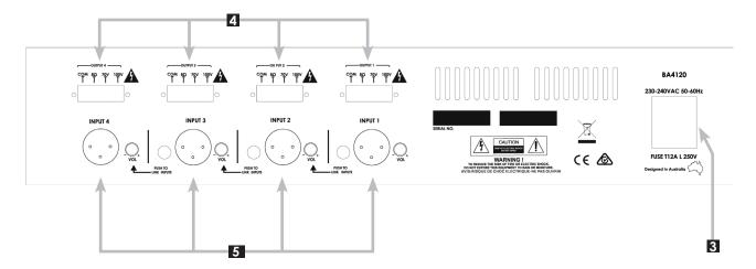
**3. Mains Socket:** The unit is connected to the mains circuit with a standard IEC type power lead. This socket contains a rated slow blow fuse.
