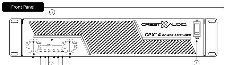
1 The CPX 4 amplifier has a combination AC switch/circuit breaker on the front panel. If the switch shuts off during normal use, push it back to the ON position once. If it will not stay on, the amplifier needs servicing.
