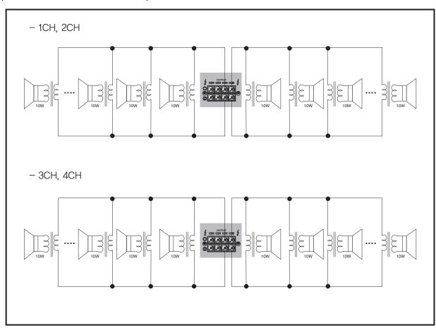
\* Caution: 1. Make sure that the total impedance does not equal or less than the rated impedance.
