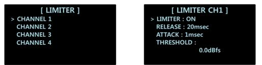
In LIMITER settings, you can set up each channel differently.
