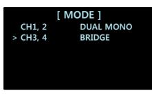
In MODE settings, you can select 5 different modes: DUAL MONO, STEREO, BI-AMP 1, BI-AMP 2, and BRIDGE. Initially, CH1, 2, 3, 4 are all set to DUAL MONO.
