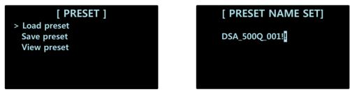
PRESET settings offers Load preset, Save preset, and View Preset functions. Instructions for PRESET settings are identical to the instructions for PRESET settings from the IN MENU. For more detailed setting instructions, please refer to section 4. 5 PRESET SETTING on page 17 of this manual.
