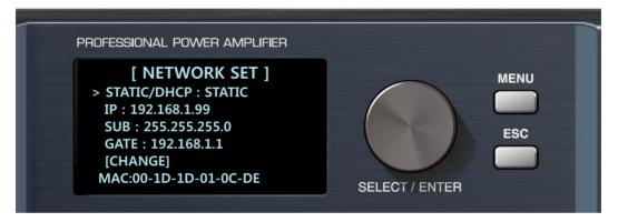
In NETWORK SETUP, you can check the NETWORK specifications of the current device.
