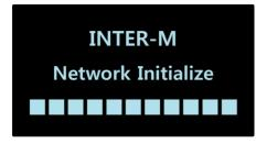
This initial screen appears when the power cable is connected to the set and the DSP begins to boot up. If indicates that the device is currently booting up. Boot-time is approximately 10 seconds.
