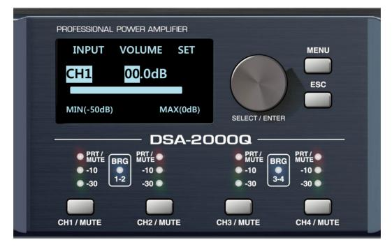
You will be redirected to this screen if you press the CH/MUTE button from the initial OLED screen. You can turn the SELECT/ENTER (ENCODER) dial left/right to control the volume.
