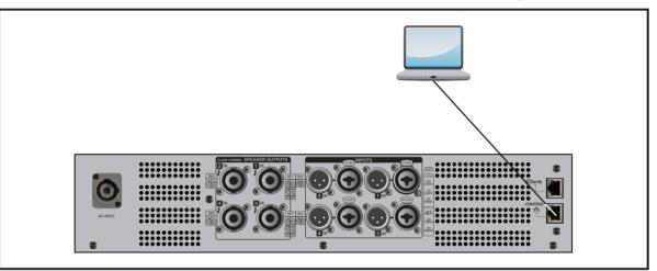
• How to connect your PC with 2 or more devices Connect the ETHERNET PORT on the back of the device and the ETHERNET PORT on your PC using a HUB.
