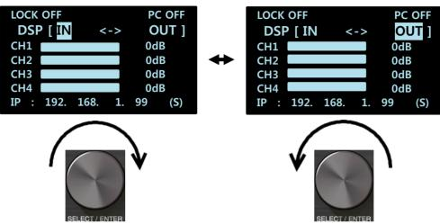
If you press down the SELECT/ENTER (ENCODER) dial after navigating to the item you want to adjust, you will be redirected to the sub-settings of the particular item. You can adjust the GAIN for each channel between -50.0dB and 00.0dB. You can change the integer and the decimal points separately. Also, the integer and decimal points that can be adjusted will be highlighted with a white background as shown in the above image.
