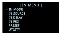
The IN MENU features multiple items including IN MODE, IN SOURCE, IN DELAY, IN PEQ as well as PRESET and UTILITY. PRESET, UTILITY items are also available in the OUT MENU.
