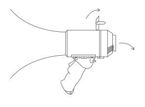
(2) INSERT 8 x AM2 C SIZE BATTERIES (NOTING BATTERY POLARITY IN HOLDER). REPLACE COVER AND RE-CLIP LATCH. (BATTERIES NOT INCLUDED)
