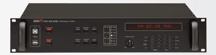
PW-6242B is a program timer device that users can set a certain date and time to perform a scheduled broadcast in 6000 system. A user can upload or download the files in PC to the inserted SD card by connecting a USB cable, and also can copy the sound source stored in the USB memory to the SD card. In addition, scheduler set up can be easily done through a management program by connecting PC.
