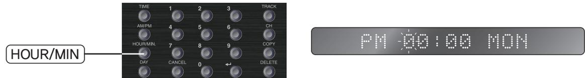
4) If pushing HOUR/MIN button once again, MIN flashes on display window and input MIN using digit button. Whenever pushing the button once, TIME and MIN setting status converts and if pushing HOUR/MIN button under MIN status, you can set up SEC.
