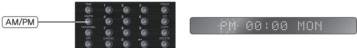
3) If pushing HOUR/MIN button, TIME flashes on display window and input time using digit button.
