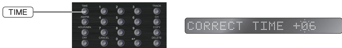
2) Input the setting value with digit button. You can set within the range of -12~+12 and be cautious that calibration time may change depending on the change of surrounding temperature.
