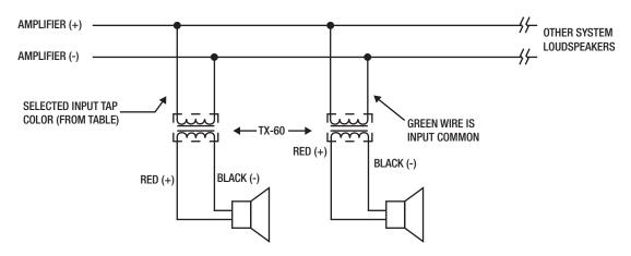
Remember to clip and insulate unused input wires; shorting any input wire to another will reduce the volume level and place an unexpected load on the power amplifier.
