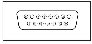
You can use conveniently Remote Control (Speaker zone can be selected and chime can be operated) through the D-SUB jack (15 pin)
