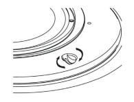
**Step 4:** Select 70V, 100V or 8 ohm bypass tapping via tapping rotary switch on front speaker baffle plate.
